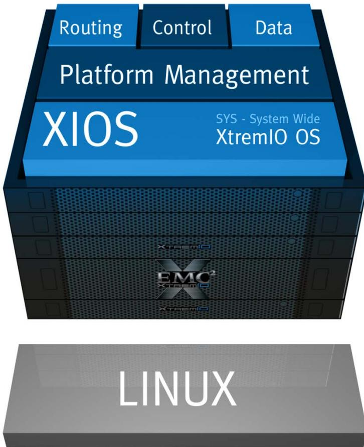
Figure 5. XtremIO Storage Controller Software Block Diagram
